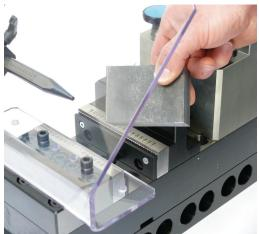
Lang's patented 'Form Closing' technology is at the heart of the system, and consists of holding teeth and depth stops arranged in a crenulated pattern 0.2mm deep. Clamping is restricted to just 3mm of the workpiece, which is retained securely by the matching holding teeth in both the billet and the vice jaws. Closing
